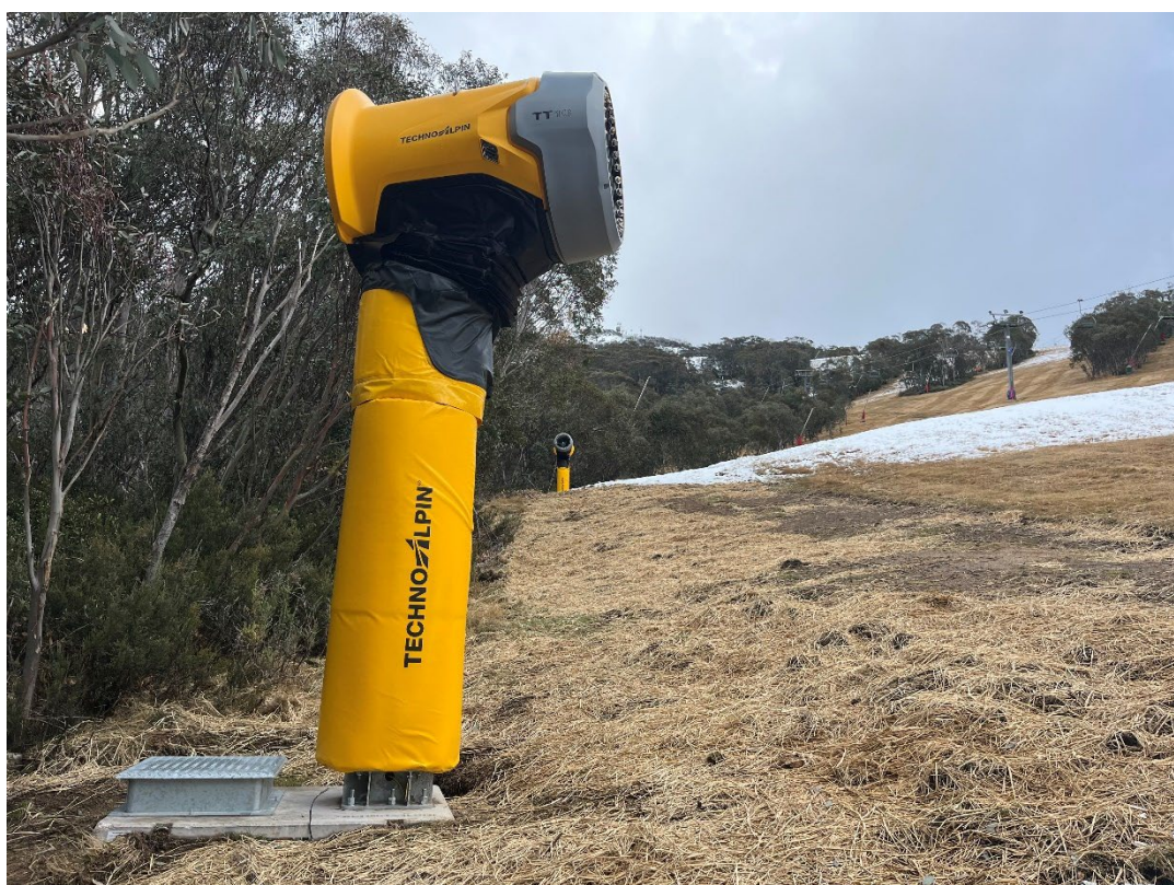
Figure 4: Example of TT10 Fan Gun and Fan Pit
